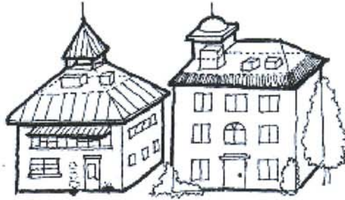
Figure 29. Examples of Screening Mechanical Equipment
